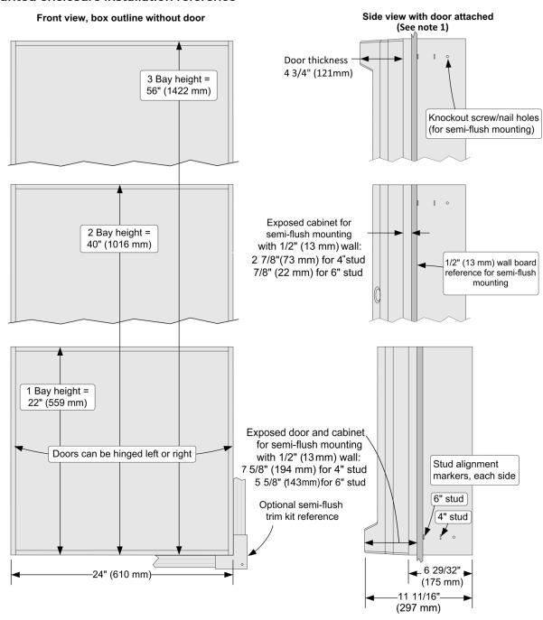
Figure 4: Installation reference
